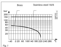
Permissible media pressure on the sensor pocket as a function of temperature
